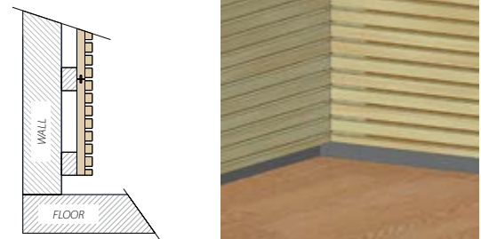
A detail of finishing the acoustic panel 50 mm above the floor
