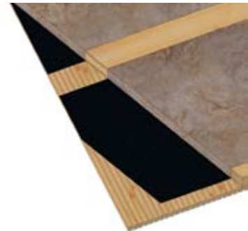
MARILYNE – detail with fibertex 75 g/m 2 + Steico Flex thickness of 50 mm from the reverse side of the panel
