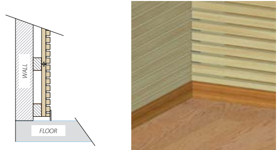
Detail of finishing with a slat
