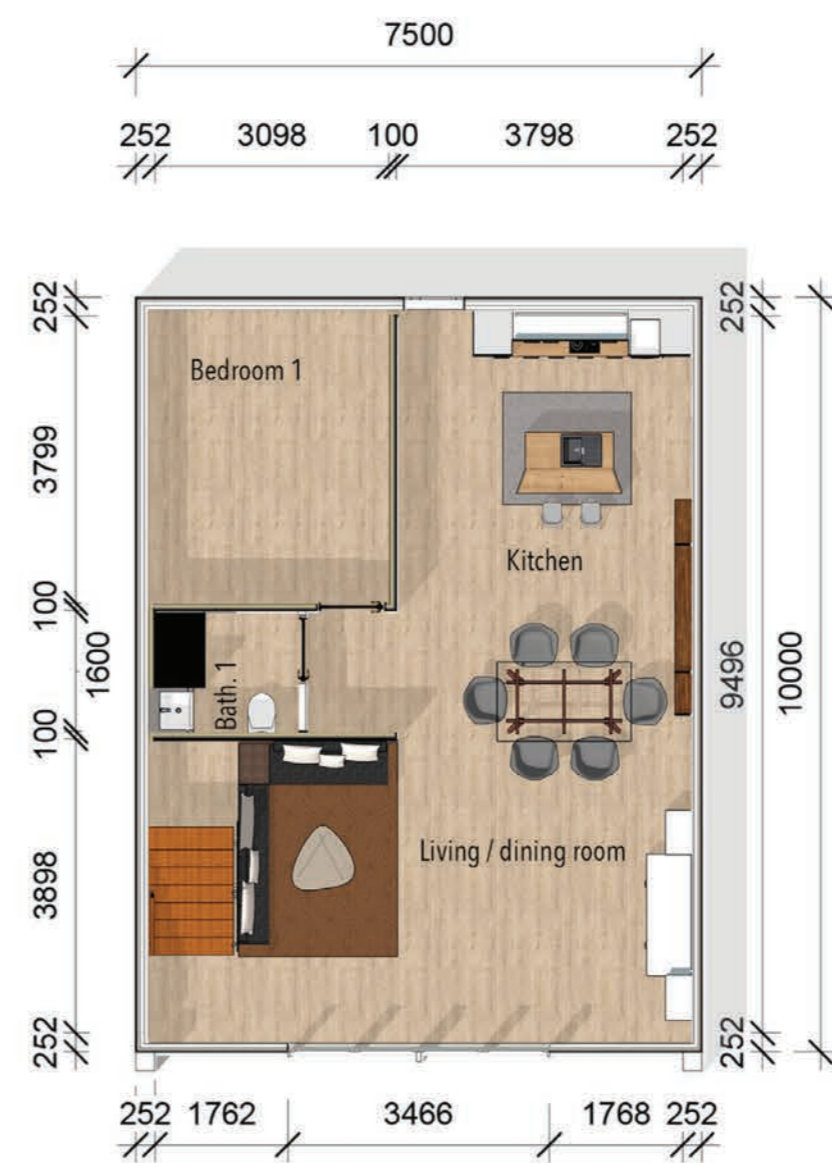
DUPLEX UNIT : GROUND FLOOR PLAN SCALE 1:100
