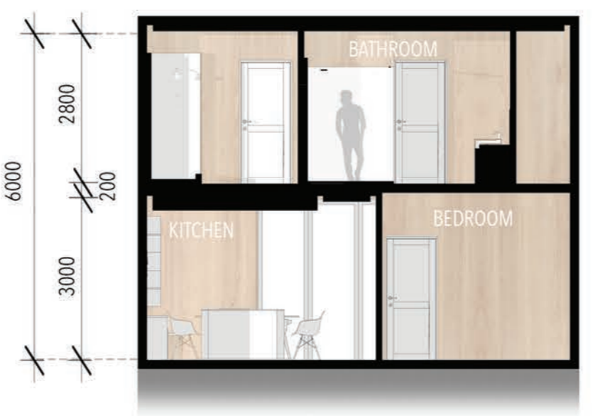
2 BED UNIT : CROSS SECTION SCALE 1:100
