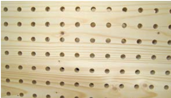
Profile made by perforation
