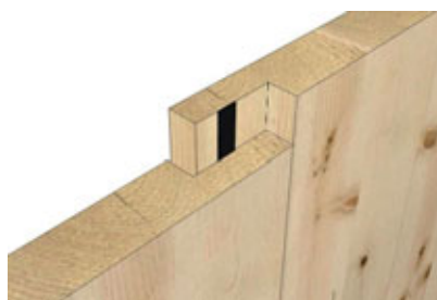
DETAIL OF A LONGITUDINAL JUNCTION 62 - WITH OVERLAP / Detalle de junta longitudinal 62 - con junta recubierta
