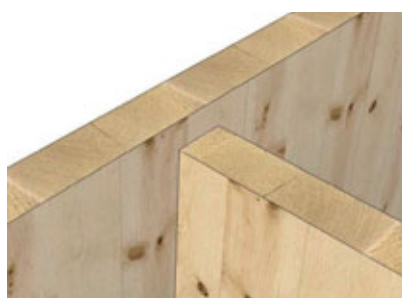
DETAIL OF A LONGITUDINAL JUNCTION 62 - WITH OVERLAP / Detalle de junta longitudinal 62 - con junta recubierta
