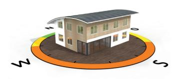
Depending on location and orientation of a building, its facade surfaces are exposed to different stresses, which change the appearance of the building. In addition to the weather effects, geographic location, altitude
