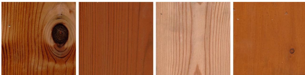
Figure 2: Test samples (from left: thermally modified pine untreated and treated, Siberian larch untreated and treated)
