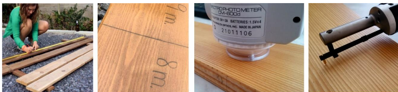
Figure 3: The test samples marking and measurements using spectrophotometer and profilometer (from left)
