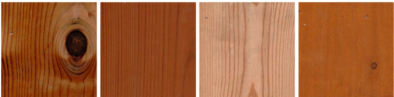
Figure 14: Test samples (from left: thermally mod. pine untreated and treated, Siberian larch untreated and treated)
