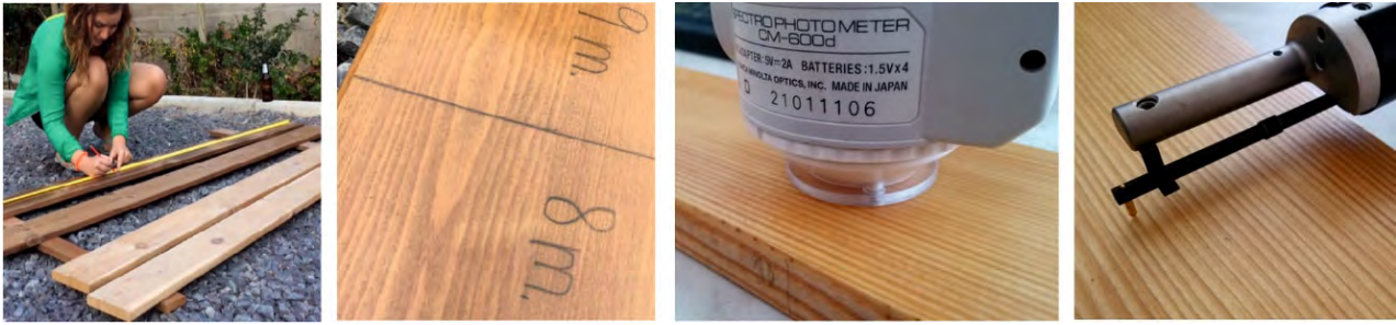
Figure 15: The test samples marking and measurements using spectrophotometer and profilometer.
